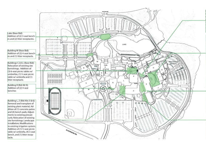
Buildings F,X (Bid Alt3): Removal of existing plant material, Addition of two concrete bench pads; Landscape installation; Modifications to existing irrigation system; Addition of (2) 3-seat benches.
