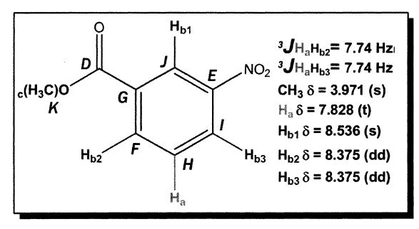
Figure 2-1. Correspondence with the <sup>1</sup>H-NMR and <sup>13</sup>C-NMR spectra. In this Figure, [b1, b2, and b3] are overlapping signals in the spectrum and are labeled to reflect that. J coupling constants are also listed.
