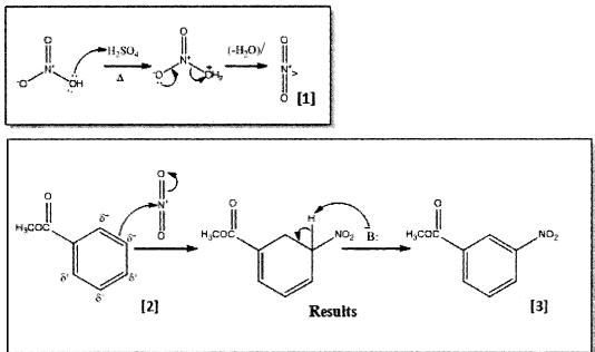
Figure 1-2. Mechanism for the *meta*-directed attack of the nitronium ion.
