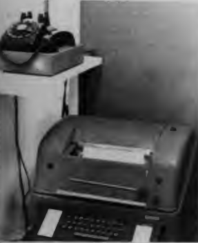
The teletype machine in the Hearing Impairment office allows the deaf to use the telephone.
