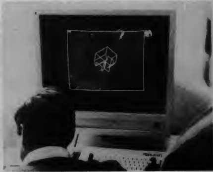
Engineers can see their concepts come to life within a few seconds. Tests may be conducted for mechanical stress, heat, motion and pressure. Wind tunnel testing can be duplicated in some CAD programs. CAM can translate the design into punched tapes. The tapes are fed into numerically controlled tools, which produce the parts as specified in the design. Photos by Bob Niek.
